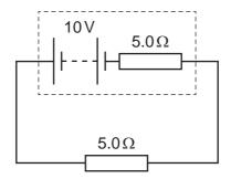
Which change occurs when the  $5.0\,\Omega$  load resistor is replaced with a  $50\,\Omega$  load resistor?
