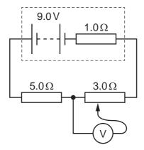
The sliding contact of the potentiometer is moved over its full range of movement.
